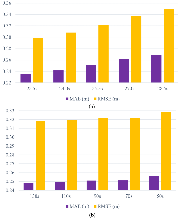
Fig. 9. The prediction errors measured by MAE and RMSE using upstream wave information for different lengths of the (a) output time horizon and the (b) input time horizon.
